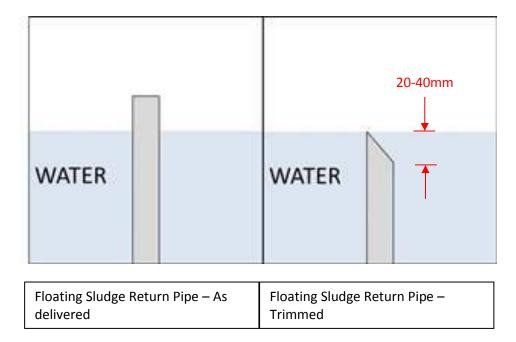
The FSR pipe must be trimmed as shown above. Ideally this should be done with pipe shears, not a saw, to ensure a clean cut.
