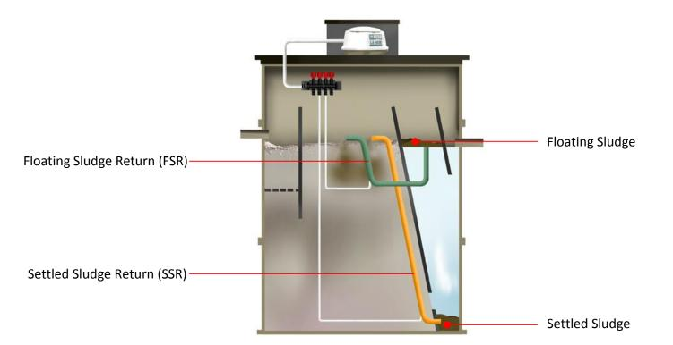
The Floating Sludge Return (FSR) pipe in the Clarification Chamber must be trimmed so that it is able to skim the surface of the water. This can only be done once the tank is full of water. Please see the pictures below.
