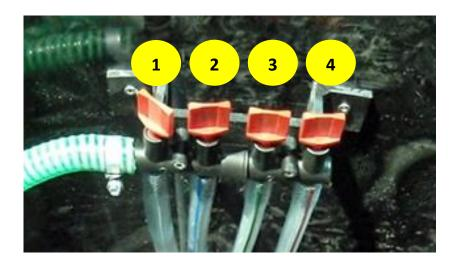
When the tank is supplied the airline to the FSR is not connected to valve 2. The FSR airline should be cut to length and attached to valve 2.
